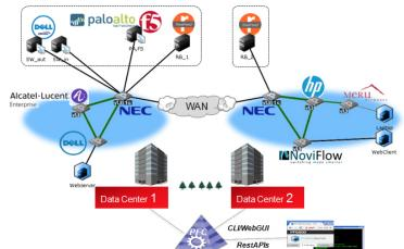
Figure 2-2: Service Chaining over the WAN (Physical Topology)
