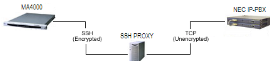
Figure 6-1 SSH Encryption Between MA4000 and IP-PBX
