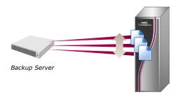
HYDRAstor's Express I/O is a lightweight data transfer protocol that delivers more efficient data transfer than standard protocols such as NFS and CIFS. Express I/O reduces the overhead of data access and maximizes backup performance. With Express I/O, backup servers can achieve maximum performance with HYDRAstor resulting in shorter backup windows.
