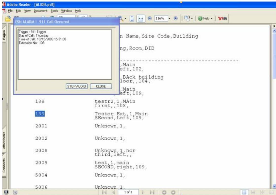
**NOTE:** The Alarm application keeps polling the database server in the configurable interval that can be configured in the 'ESNAlarmClient.ini' file.
