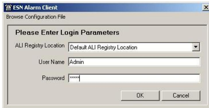
Enter a username and password of ESN Alarm user to login to the E911 Alarm client application once you have selected the ALI Registry location details. If the login is successful, you will see a telephone icon sit in the system tray as shown in the image.
