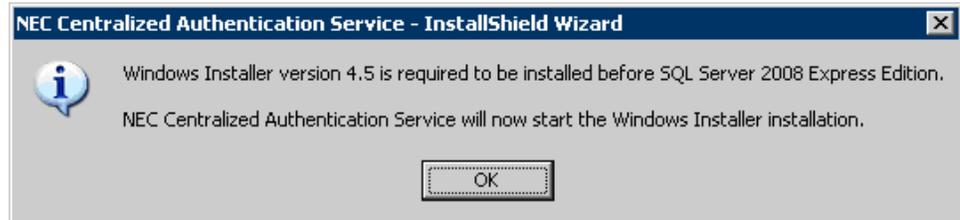
—Click **OK**. [Figure 4-6](#) displays when the Windows Installer 4.5 installation completes.
