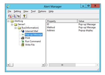
Set for each alert to be displayed on the tree. Setting results are listed on the right side of the tree.
