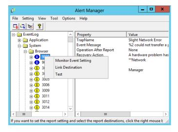
The test enables users to verify whether each event displayed on the tree is notified to the associated destination by generating an event.
