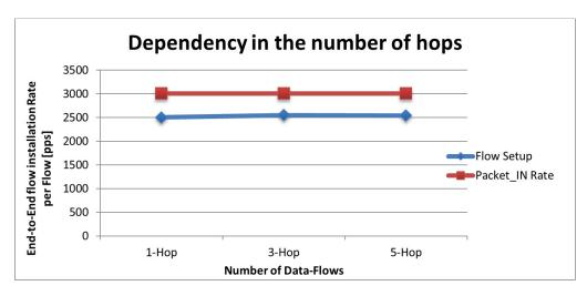
End-to-End Flow Installation Rate (pps) measurement will be performed for a varied number of data flows to measure the controller flow installation performance.
