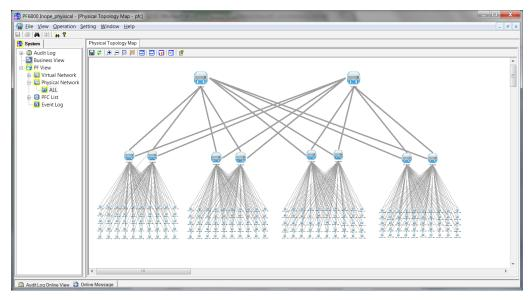
Each of the 200 small icons represents an OpenFlow switch emulated by Ixia and all links between switches are automatically discovered by the NEC Controller.
