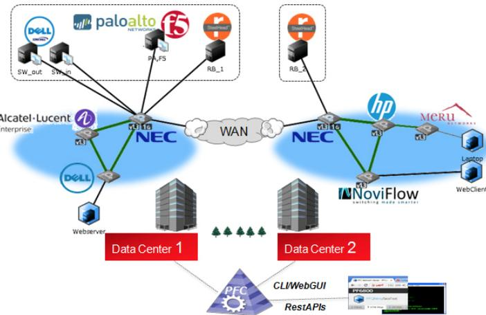
Figure 2-2: Service Chaining over the WAN (Physical Topology)
