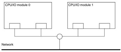
Example 2) Configure the duplex network which corresponds to multiple LAN connection.
